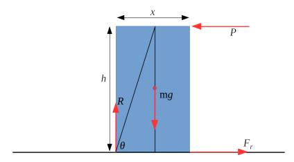
For the box to topple (or tip), the anticlockwise moments must be greater than the clockwise moment. When the block is on the point of tipping then the normal reaction force will be acting at the front corner of the block.
