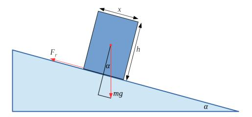
The box will start to slide when  $mg \sin \alpha > \mu mg \cos \alpha$ , so when  $\tan \alpha > \mu$ .
