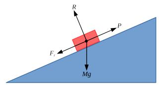
P is the "Pulling force" and  $F_r$  is the friction. At the point of moving we have  $F_r = \mu R = 0.7R$ . Resolving forces parallel and perpendicular to the slope we have:
