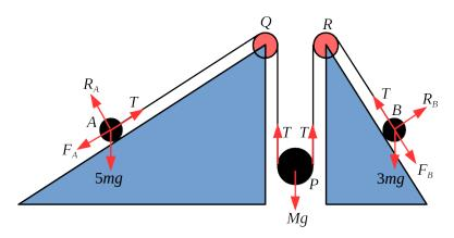
The plane with A on is inclined at angle  $\theta = \arctan \frac{7}{24}$ , i.e.  $\tan \theta = \frac{7}{24}$ , and so we have  $\sin \theta = \frac{7}{25}$  and  $\cos \theta = \frac{24}{25}$ . The plane with B on is inclined at angle  $\phi = \arctan \frac{4}{3}$ , i.e.  $\tan \phi = \frac{4}{3}$ , and so we have
