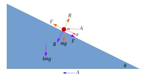
Here the forces acting on the particle are orange and the forces acting on the wedge are purple. I have called the acceleration of the wedge A. You could instead draw two different diagrams, one showing the forces and accelerations for the particle and one showing the forces and accelerations for the wedge.
