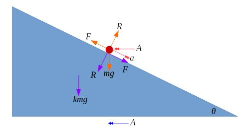
Here the forces acting on the particle are orange and the forces acting on the wedge are purple. I have called the acceleration of the wedge A. You could instead draw two different diagrams, one showing the forces and accelerations for the particle and one showing the forces and accelerations for the wedge.
