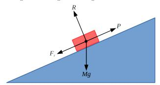
P is the "Pulling force" and  $F_r$  is the friction. At the point of moving we have  $F_r = \mu R = 0.7R$ . Resolving forces parallel and perpendicular to the slope we have:
