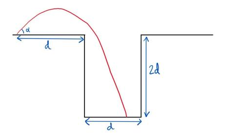
(i) (a) Let the initial position of the particle be at (0,0). This horizontal displacement of the particle is given by  $x = vt \cos \alpha$  and the vertical displacement is given by  $y = vt \sin \alpha - \frac{1}{2}gt^2$ . The time when the horizontal displacement is equal to d is given by:
