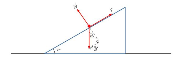
If the particle is in equilibrium then resolving parallel and perpendicular to the slope we have:
