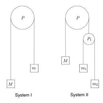
(i) For system I show that the acceleration,  $a_1$ , of the particle of mass M, measured in the downwards direction, is given by
